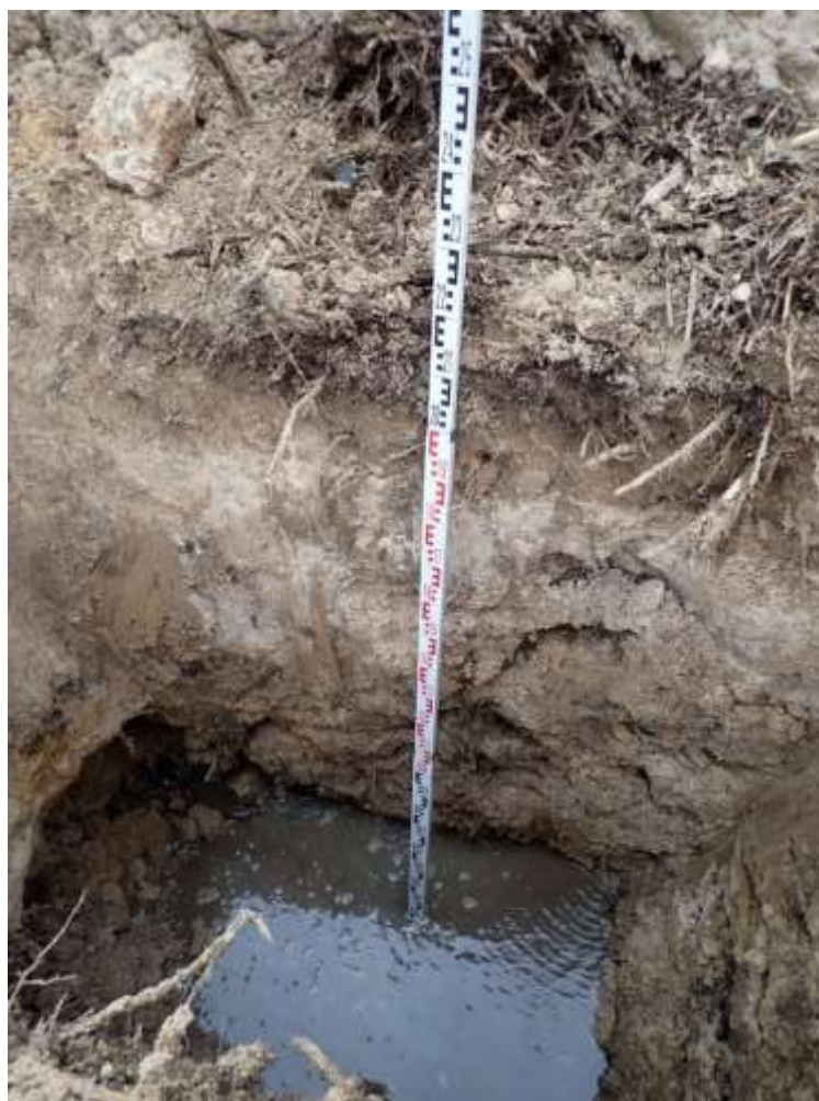
Plate 6 The porous, spongy, humus-rich calcium carbonate containing pods of organic material (relict tufa) in trial pit 4, with a topsoil of partially-decomposed organic matter, towards the southern end of the proposed LRD site, February 2025. Pods of this material occur in pockets throughout the site (see also Plate 8).
