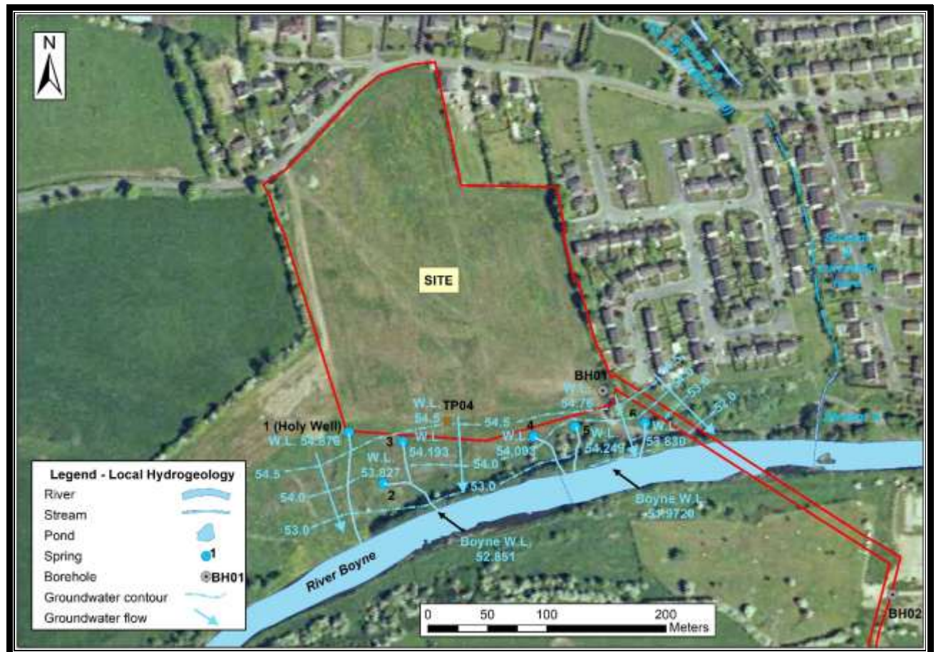
Figure 19: Water levels at springs, in the River Boyne and in BH01 and Trial Pit 04 on the proposed LRD Site, as well as interpolated groundwater contours from this, and groundwater flow directions. (O.S. Licence EN 057926).
