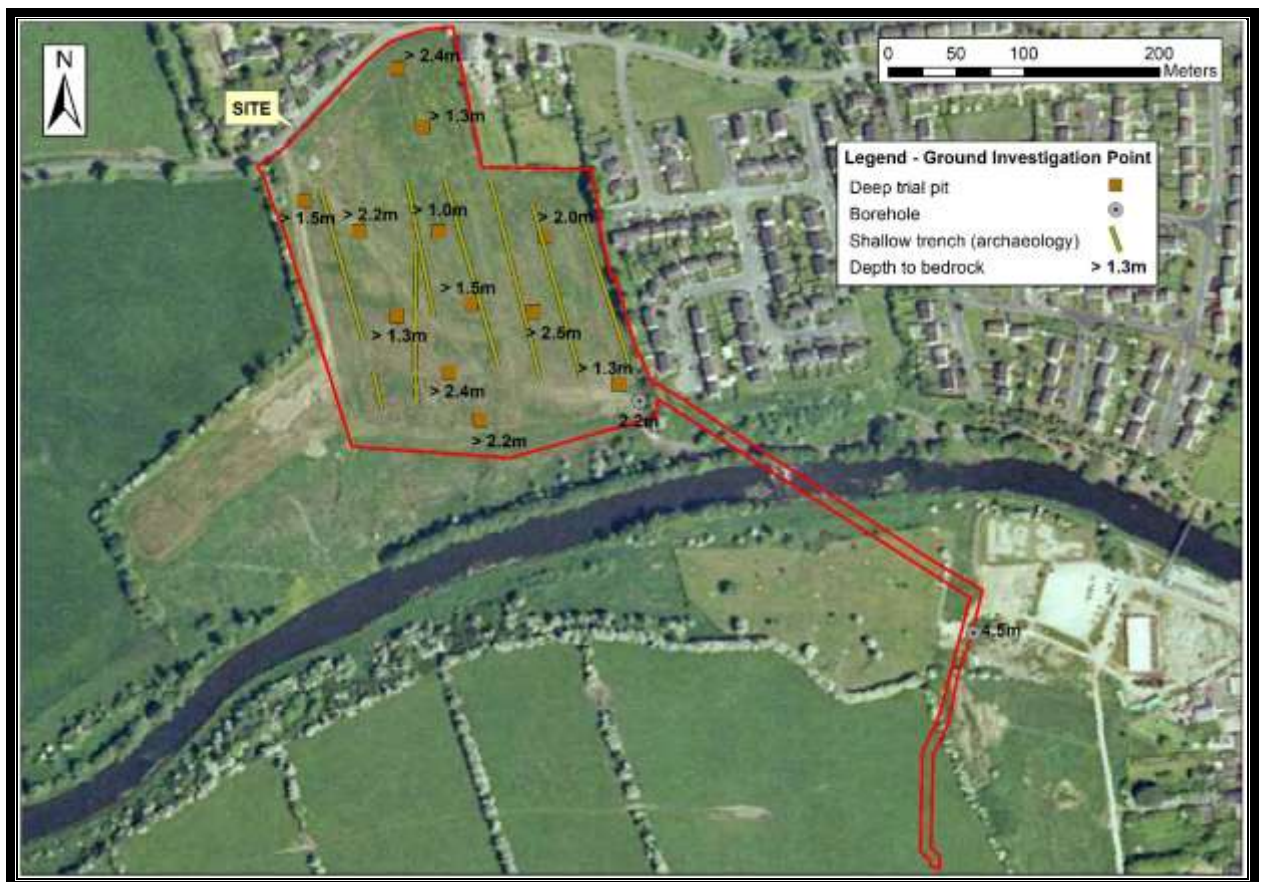
Figure 6: Point depths to bedrock at trial pit localities excavated and borehole localities drilled across the proposed LRD Site area (O.S. Licence EN 057926).
